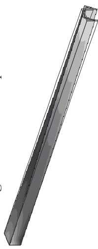
mode shape 3, \omega_3=769.5 , torsional vibr
